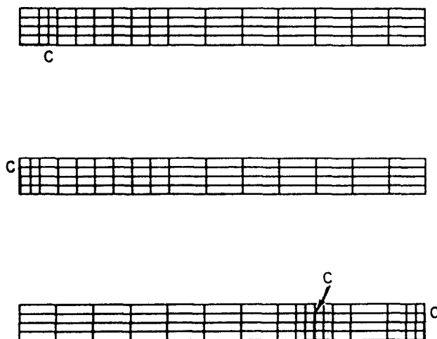
Fig. 8. One quarter of the finite element mesh of the interior regions of the three problem geometries shown in Fig. 7. C indicates the crack tip position.
